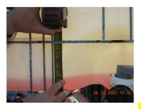
Measurements are taken on the outside of the bottle at the valve area. We chose not to measure from the filling hole (center) because that would require opening every unit with excess heel. This will require a tool, a dipstick, cleaning supplies and a collection container for contaminated rags. Measurements from the filling hole vs. the bottle exterior do not match.
